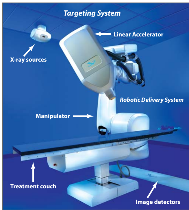
The Cyberknife Radiosurgery Device showing the components of the system
